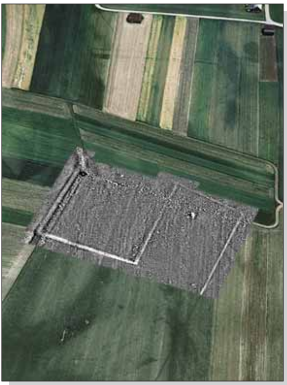
Figure 2: The combination of aerial picture and geophysical mapping need not be based on rectified aerial pictures. The image containing the results of the geophysical survey can be stretched and inclined corresponding to the inclination and orientation of the aerial picture. Celtic structures at Mengen, near Sigmaringen, Baden-Württemberg. Aerial photo by Otto Braasch
